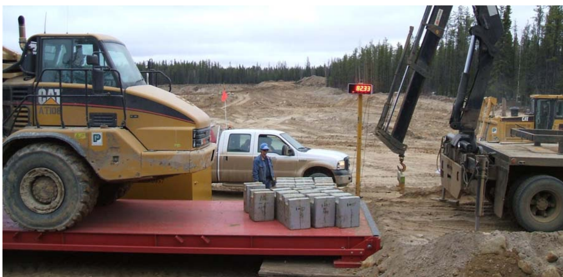
Strain Testing a Portable Truck Scale
